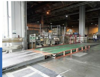
20 feet pit scale scale : 20ton
