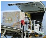
Loading/ Unloading Arriving baggage and cargo is unloaded from the aircraft before departing baggage and cargo is loaded.
