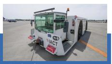
**6 Towing Cars** A vehicle for towing an aircraft
