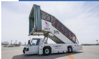
9 Passenger Boarding Steps A vehicle for crew and passenger access to an aircraft
