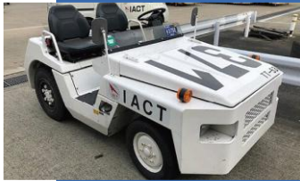
60 Towing Tractors A vehicle for towing ULD dolly and bulk cart
