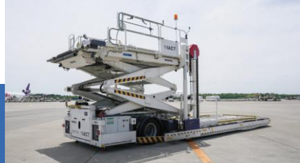
9 Main Deck Loaders A vehicle for loading and unloading ULD from a freighter aircraft's main deck
