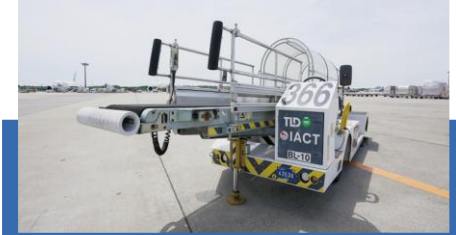
11 Belt Loaders A vehicle for loading and unloading bulk cargo and baggage from an aircraft's bulk cargo bay
