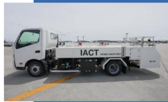
2 Water Cars A vehicle for supplying drinking water to an aircraft
