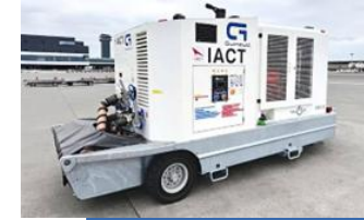
2 Air Start Units Equipment for starting aircraft jet engines
