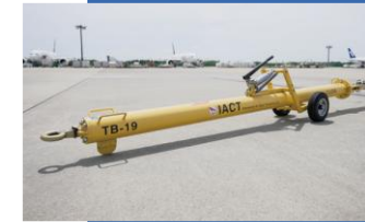
18 Tow Bars Stick-like equipment for connecting an aircraft to a towing car
