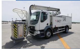
4 Deicing Cars A Vehicle for the removal of snow and ice from an aircraft
